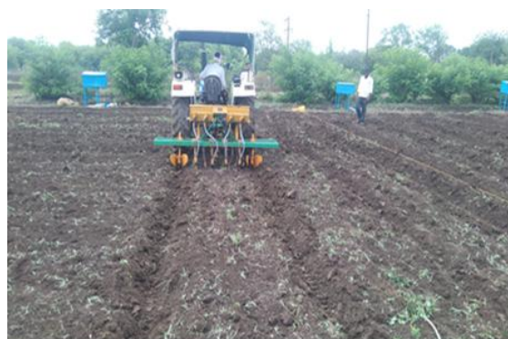
Figure 2 Land resource conservation through Broad Bed and Furrow system
